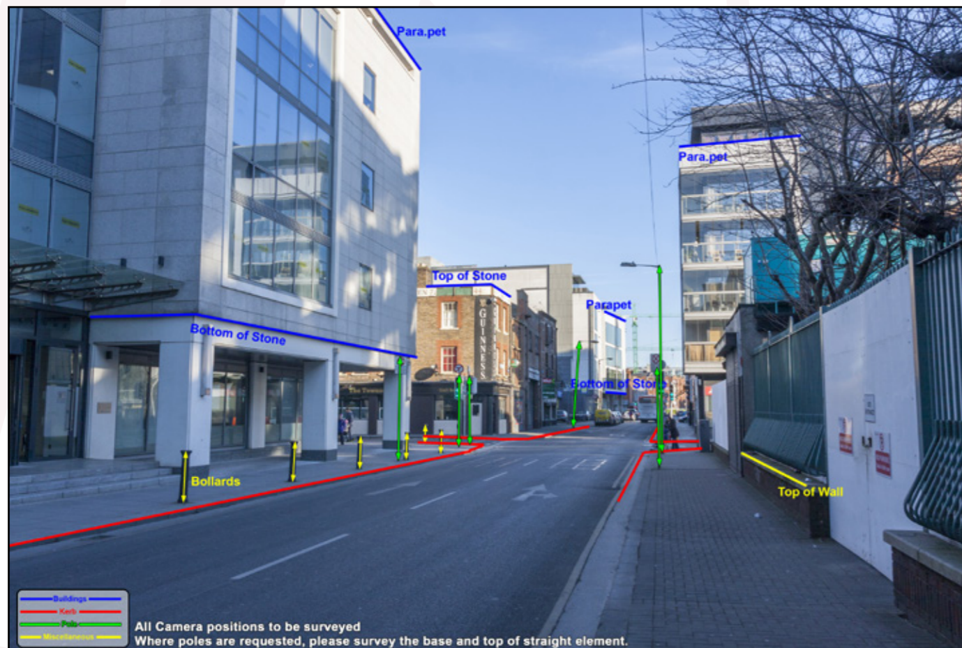
Fig.7: Fixed reference points marked for surveyour.
