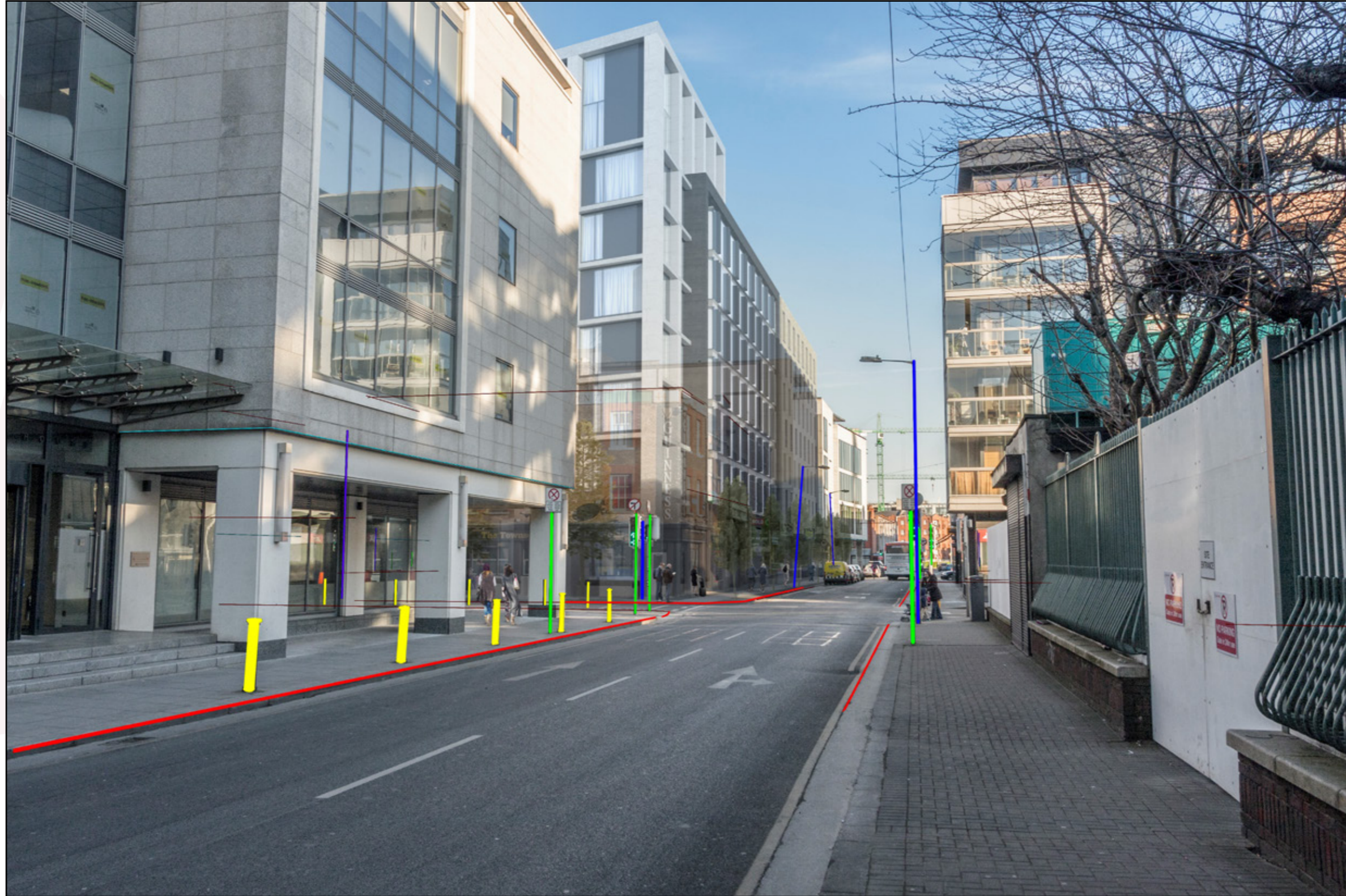
Fig.11: Fixed reference points modelled, rendered and overlaid on baseline photo confirming accuracy
