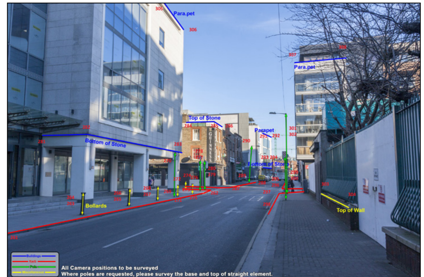
Fig.8: Fixed reference points surveyed and numbered by surveyour.
